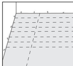
Lay the PE film, allowing at least 20cm (8") of overlap and use adhesive tape to unite.
