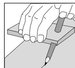
If the wall is very uneven, cut the planks with the corresponding width to eliminate the unevenness. Place the first plank on top of the second row and cut as indicated. Or draw the outline of the wall by "sliding" a cut off-piece along the wall. Then cut the planks along the line.
