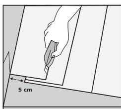
Measure and cut the planks in the last row to the correct size. Allow for a 5mm (0.2") distance to the wall. No plank should be less than 5cm (2") wide.
