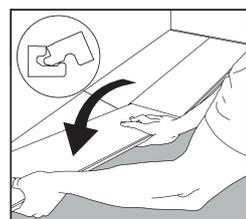
Place the short end of the plank at an angle against the previous installed plank and fold down. Ensure that the plank is positioned on the integral locking strip of the plank in the previous row.
