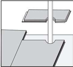
Drill the required holes in the planks, making a hole on the plank 10mm (0.4") bigger than the pipe diameter.
