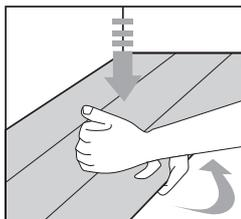
If you wish to uninstall the floor, just lift the planks a few centimetres and tap along the joint.
