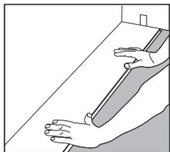
Turn the tongue side of the plank facing the wall. Maintain a gap of 5mm (0.2") on the short side.
