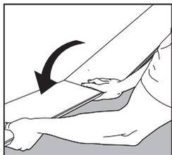
Hold the next plank against the first at an angle to the first one and lay it flat on the floor.
