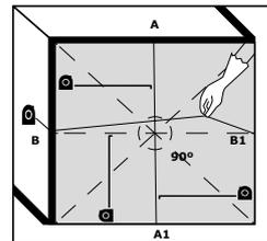
Check the wall where you are starting the installation and make sure it is squared to the opposite wall. Simply measure the room from the opposite ends of the wall to the fire wall. If measurements are different make the necessary adjustments on the first row. Draw a line using a chalk-line.
