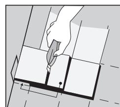
The last and first plank can be cut in the correct width. Place the last plank on top of the second to last plank. Mark the plank with the help of a piece of plank without locking the strip. Allow for 5mm (0.2") distance to the wall for the expansion gap.
