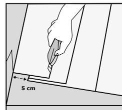
Make sure that the widths of the first and last rows planks are equal or bigger than 5cm (2") of the plank.
