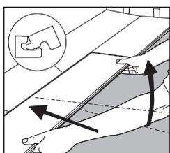
Lift the plank (together with the previous one laid in the same row) slightly up (about 30mm (1.2")), push it against the row in front and then put it down. Tip: This movement requires some gentle adjustments on the pressing angle.
