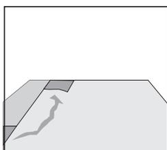
Make sure that the long sides of the planks make a straight line. Use the cut piece of the plank from the previous row to start the next one. However it must be at least 30cm (12") long. If the piece is too short, start with a new board and cut it in half. Always ensure that the end joints are staggered at least 30cm (12"). Tiles with 605 x 445 (23-7/8" x 17-1/2"), "brick" or "half brick" installation method must be used.
