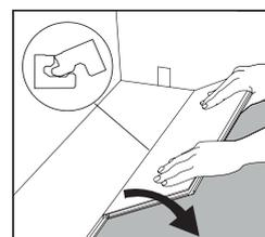
Place the first plank of the new row with the tongue side at an angle against the groove side of the plank in the previous row.
